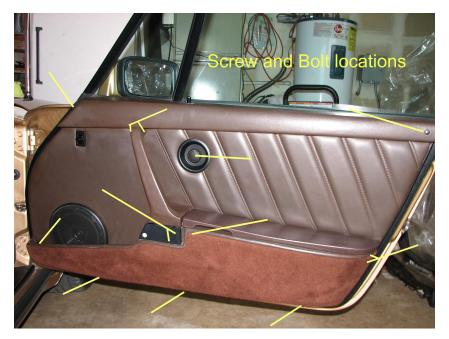
3. Remove the plug from the rear and the 2 screws from the upper sill (1 front/1 rear). Remove the trim cover from the door lock knob, retaining screw and then the knob.
